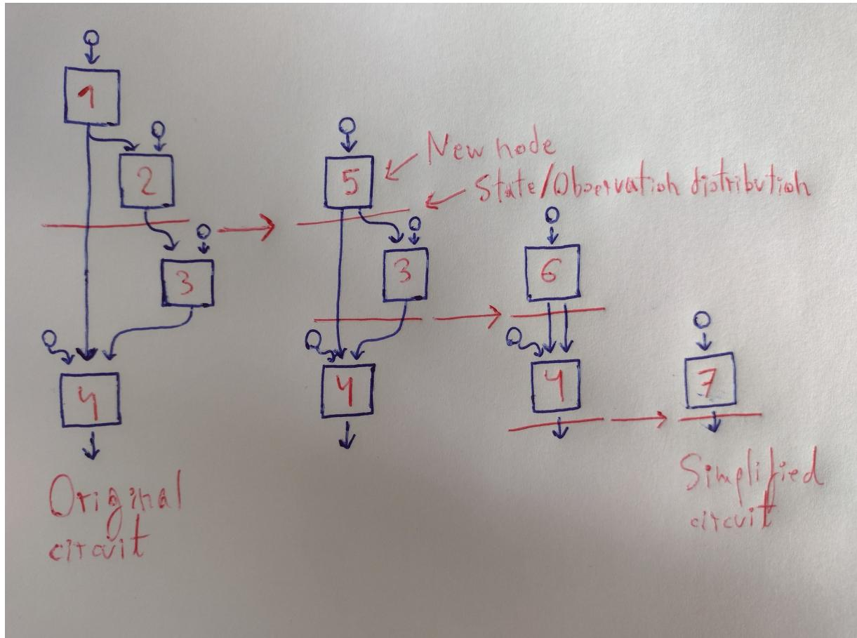
The basic idea is to take the initial circuit, along with a series of initially random circuits, and a final explicit probability distribution over the variable we care about (the reward<sup>3</sup>), and to optimize them so that the transformation between consecutive ones is as close to verifiably valid as possible. More details on this later.
